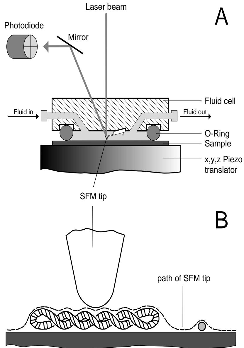
**Fig. 1.** Schematic diagram of SFM in liquid. **(A)** Cross section of the fluid cell. **(B)** Path of the tip during the scanning process. To the left a scheme of a superhelical plasmid is shown and to the right a cross section through the DNA double helix is presented. The large size of the tip as compared to the dimensions of the DNA double helix leads to an apparent DNA width in the image that is larger than the true DNA double helix diameter.
