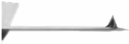
Figure 2.5 Commercial available etched silicon probe for AFM tapping mode. High magnification of an ultra sharp RTESP-probe from Veeco-Europe. The opening radius for the tip is typically below 10 nm. The resonance frequency is around 300 kHz.
