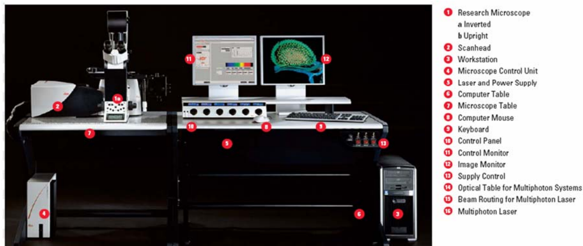
Figure 3.2: Confocal laser scanning microscope Leica TCS SP5. Image adapted from Leica TCS SP5 brochure – technical data, Leica Microsystems CMS GmbH, Mannheim ( www.leica-microsystems.com ).
