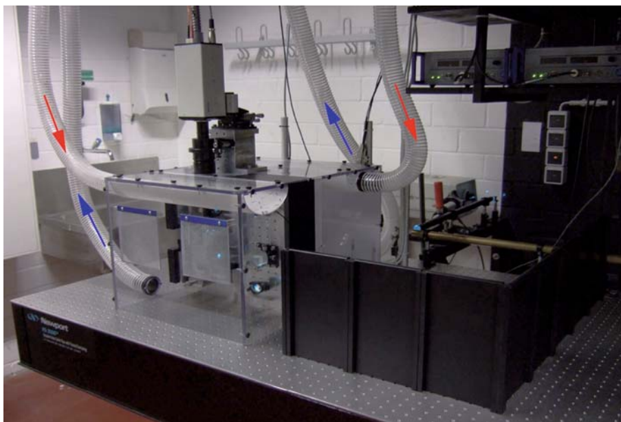
Figure 5. Photograph of the Vertico-SMI with closed incubator chamber. The red arrows (oriented downwards) indicate the supply with heated air and the blue arrows (oriented upwards) the transportation back to the temperature control unit, thus completing the cycle.
